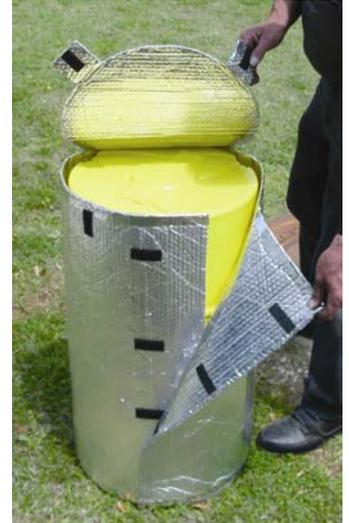
Portable sampler in an insulative wrap.
