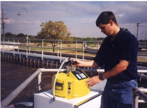
Stationary sampler on refrigerator.
