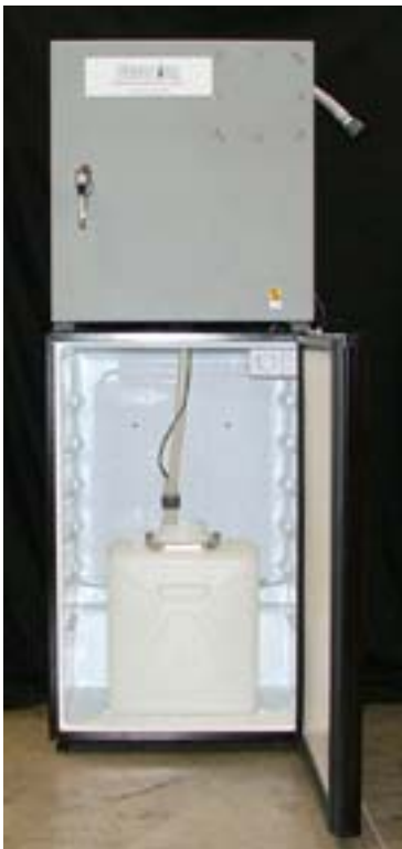
Manning Model S-5000 Sampler on an 4.9 cu. ft. Refrigerator
