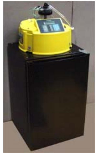
Manning Model VSR Sampler on an 4.9 cu. ft. Refrigerator
