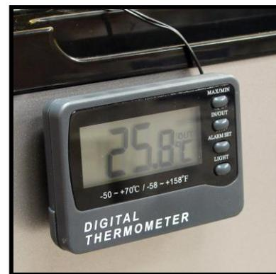
The sample sensor is located in a bottle of glycerin mounted on the lower right inside of the refrigerator to represent the eventual temperature of the sample. If desired, the sample sensor may be placed inside the sample container to display the actual temperature of the sample.
