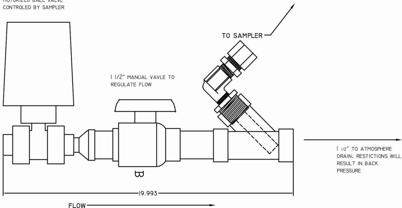
**Flow-through Cell: High Flow Setup**
