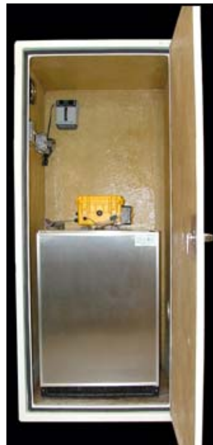
YB8 Sampler in NEMA3R Enclosure with heater and fan options.
