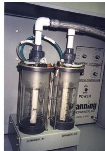
S-5200 Dual Measuring Chambers
