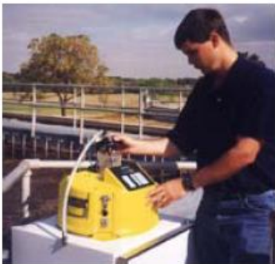
VSR Sampler Operation
