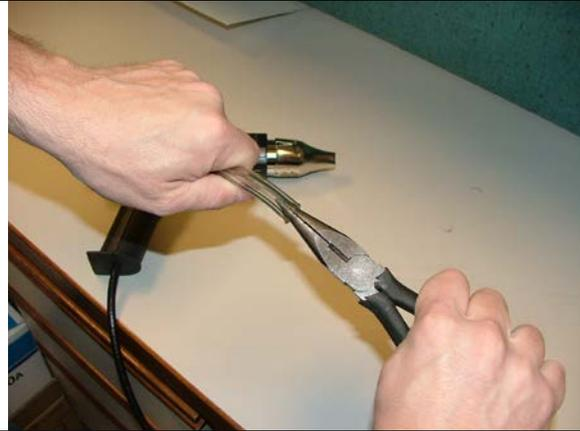
Insert a pair of round-nose pliers into the end of the hose.
