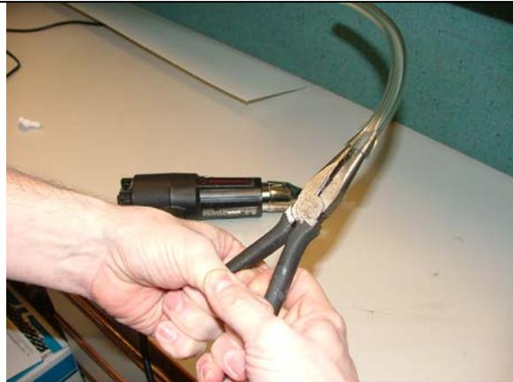
Stretch out the hose with the pliers. Rotate the pliers 90 degrees in the hose and stretch again.
