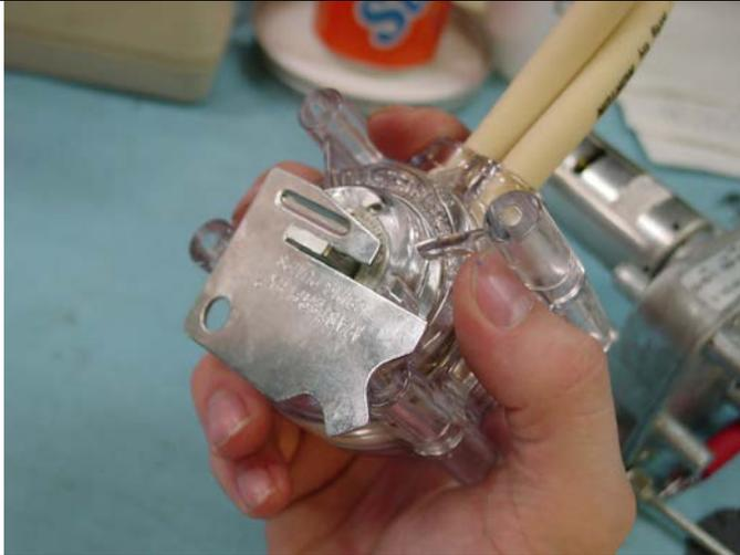
Hold two halves together and rotate rollers clockwise using the pump tool.
