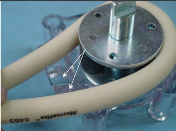
Place hose around pump rollers, making sure to place hose into grooves.
