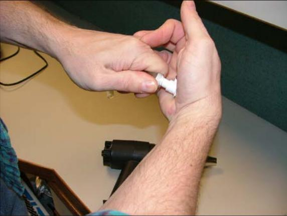
Press the fitting into the hose using a wiggling motion.
