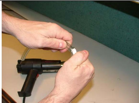
Quickly remove the pliers and insert the fitting into the end of the hose.
