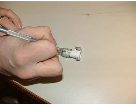
Using a knife, cut a slit in the hose along the side of the connector.
