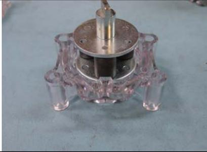
Orient rollers in 1/2 of pump housing as in picture.
