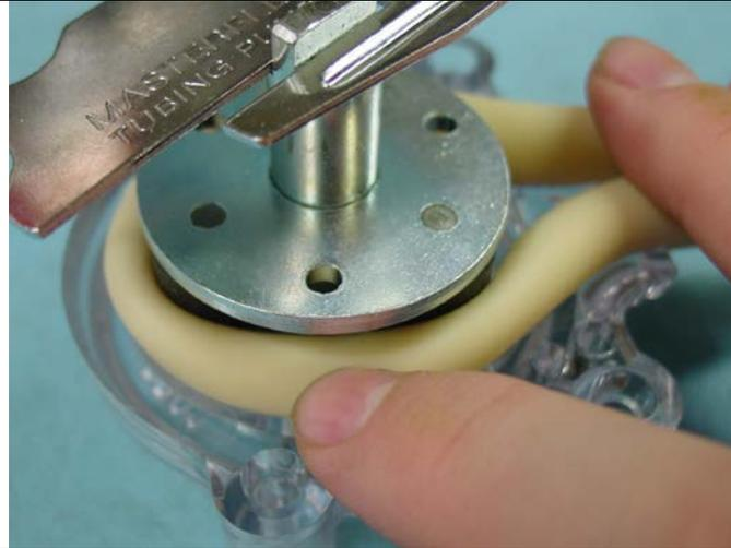
Using the pump tool\* included in the pump kit, rotate rollers clockwise while pressing hose in gap between rollers.
