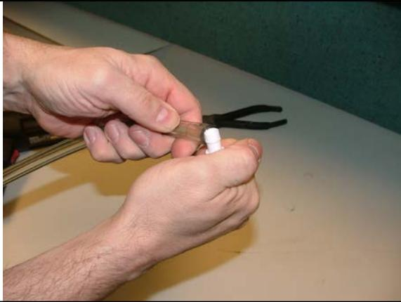
Remove fitting using a wiggling motion.
