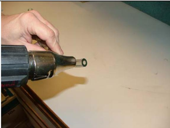
End of intake hose should be cut clean and straight.
