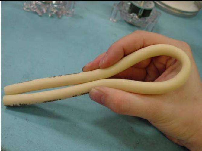
Fold pump hose in half, aligning ends and forming loop at other end.
