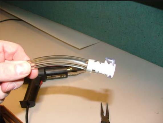
Make sure that barbed end of fitting is fully inserted into hose
