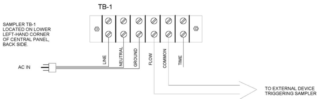
Figure 7. S-5000 Electrical Connections
