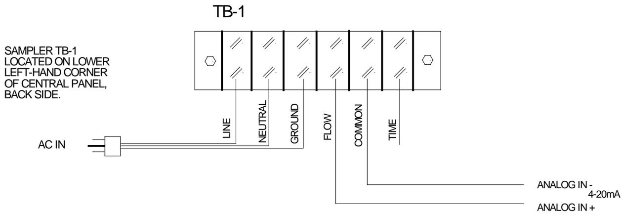
Figure 14. S-5000 Analog (4-20mA) Connections
