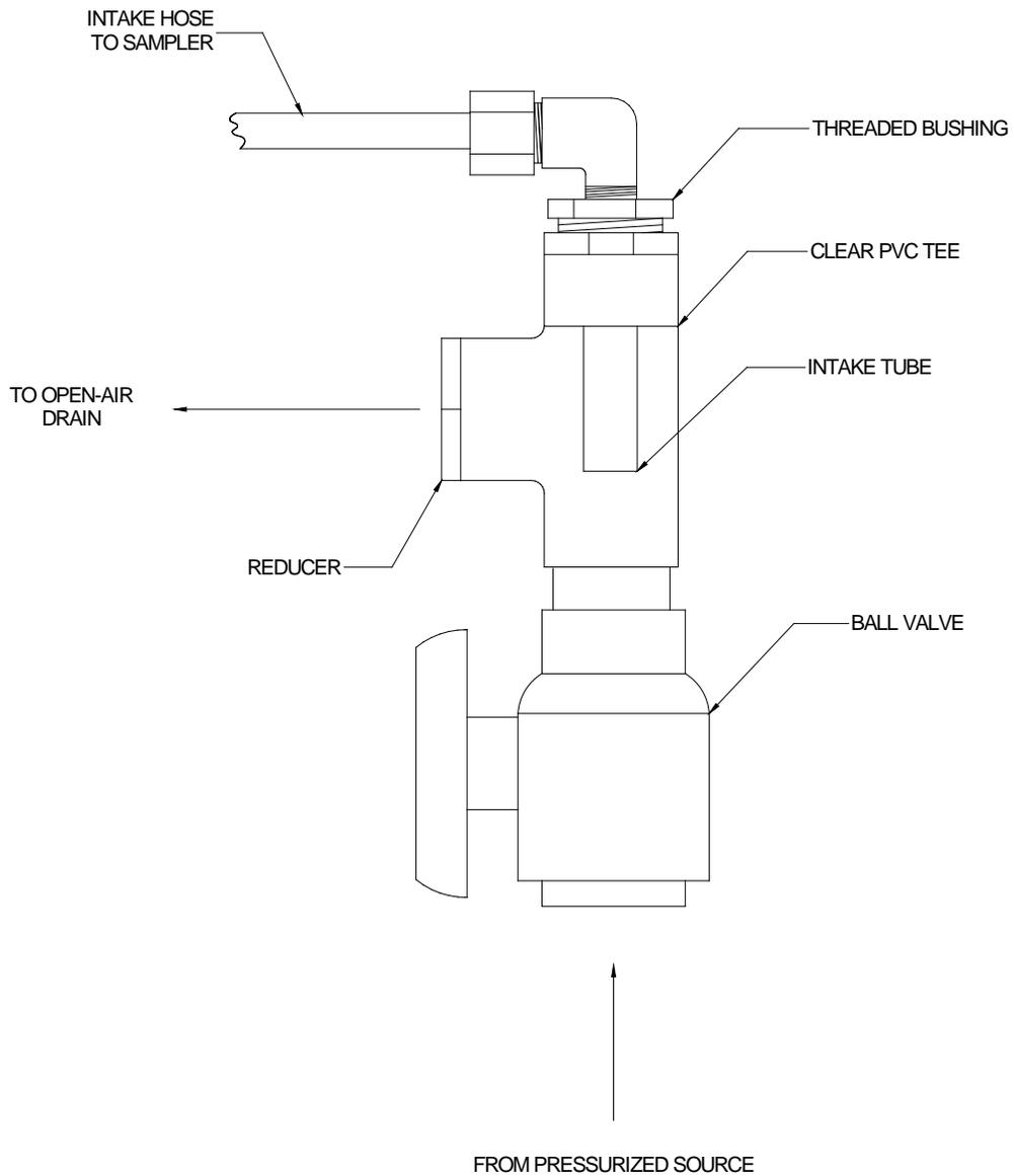
**Figure 17. Flow-Through Cell Operation**
