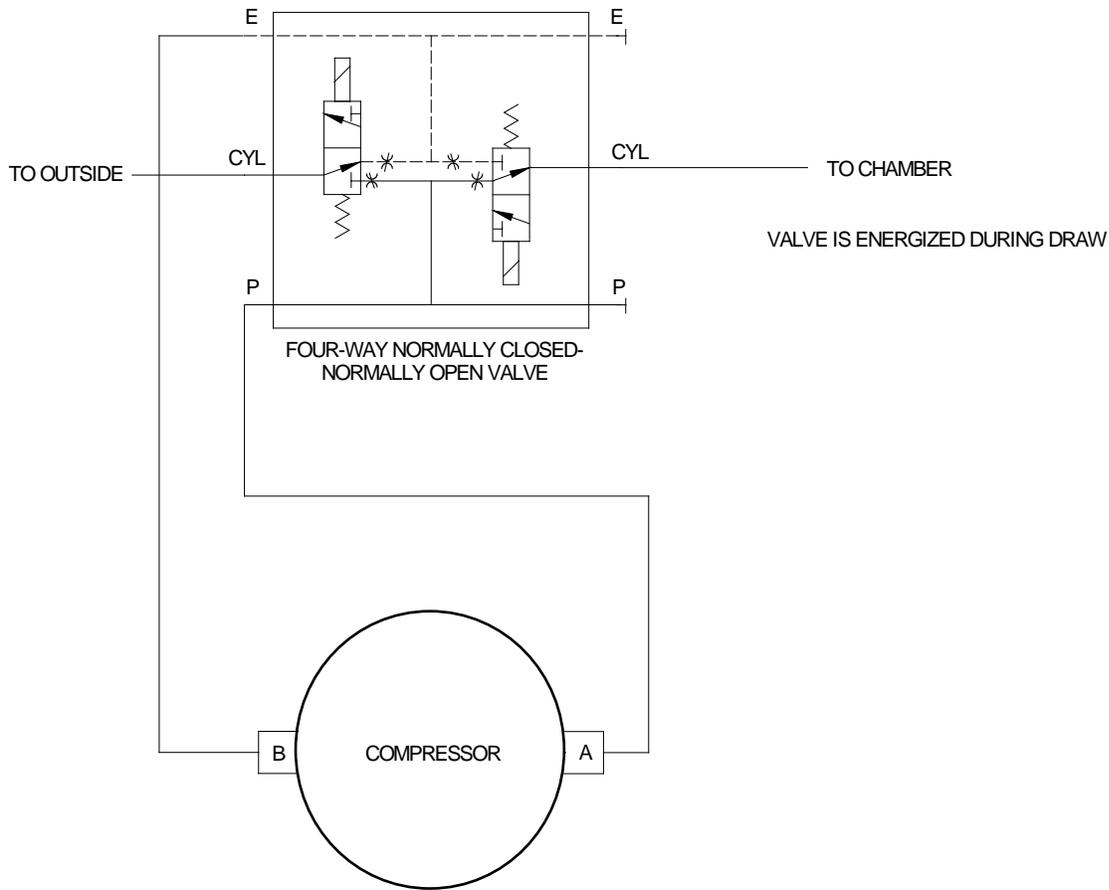
Figure 22. S-5000 Air System Diagram (Jan 2014 and Earlier)
