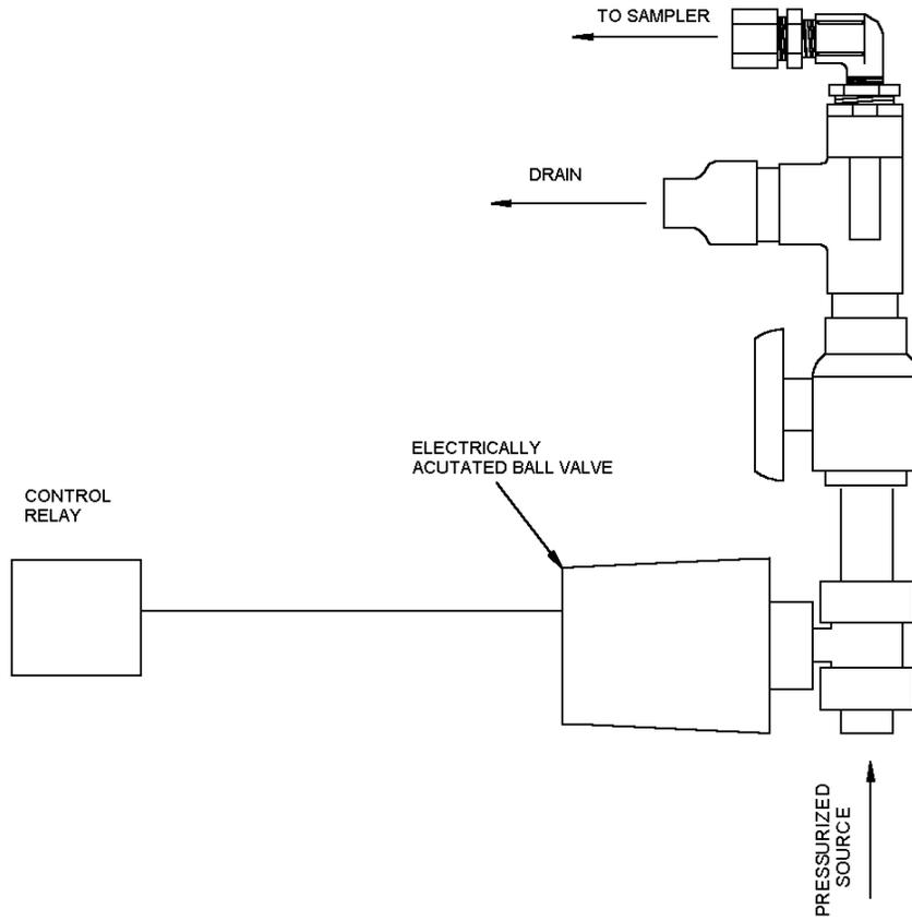
Figure 18. Flow-Through Cell with Electrically Actuated Ball Valve
