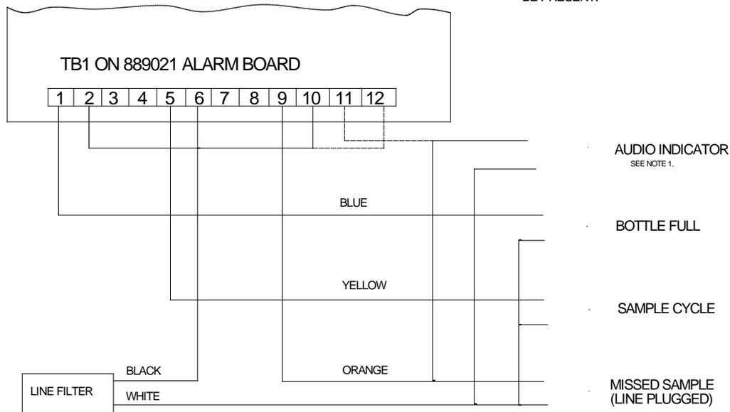
**Figure 12. Typical Alarm Board Wiring**
