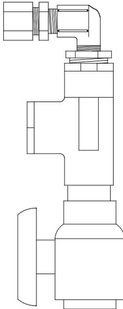
**Figure 16. Flow-Through Cell**
