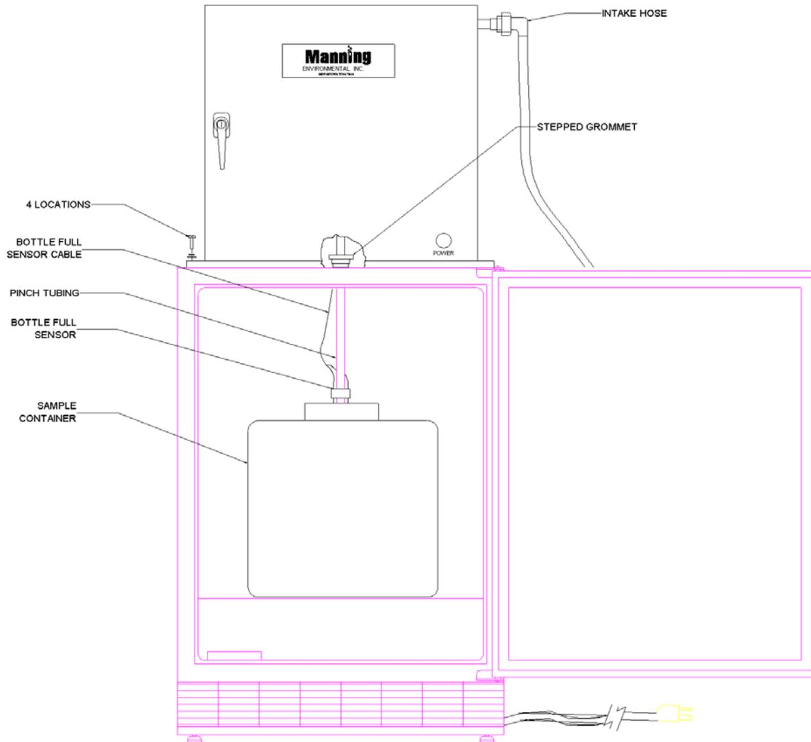
Figure 10. Model S-5000 Sampler Installation with Refrigerator
