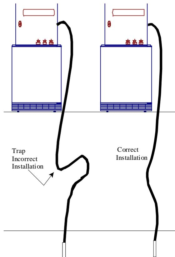
**Figure 8. Intake Hose Placement**
