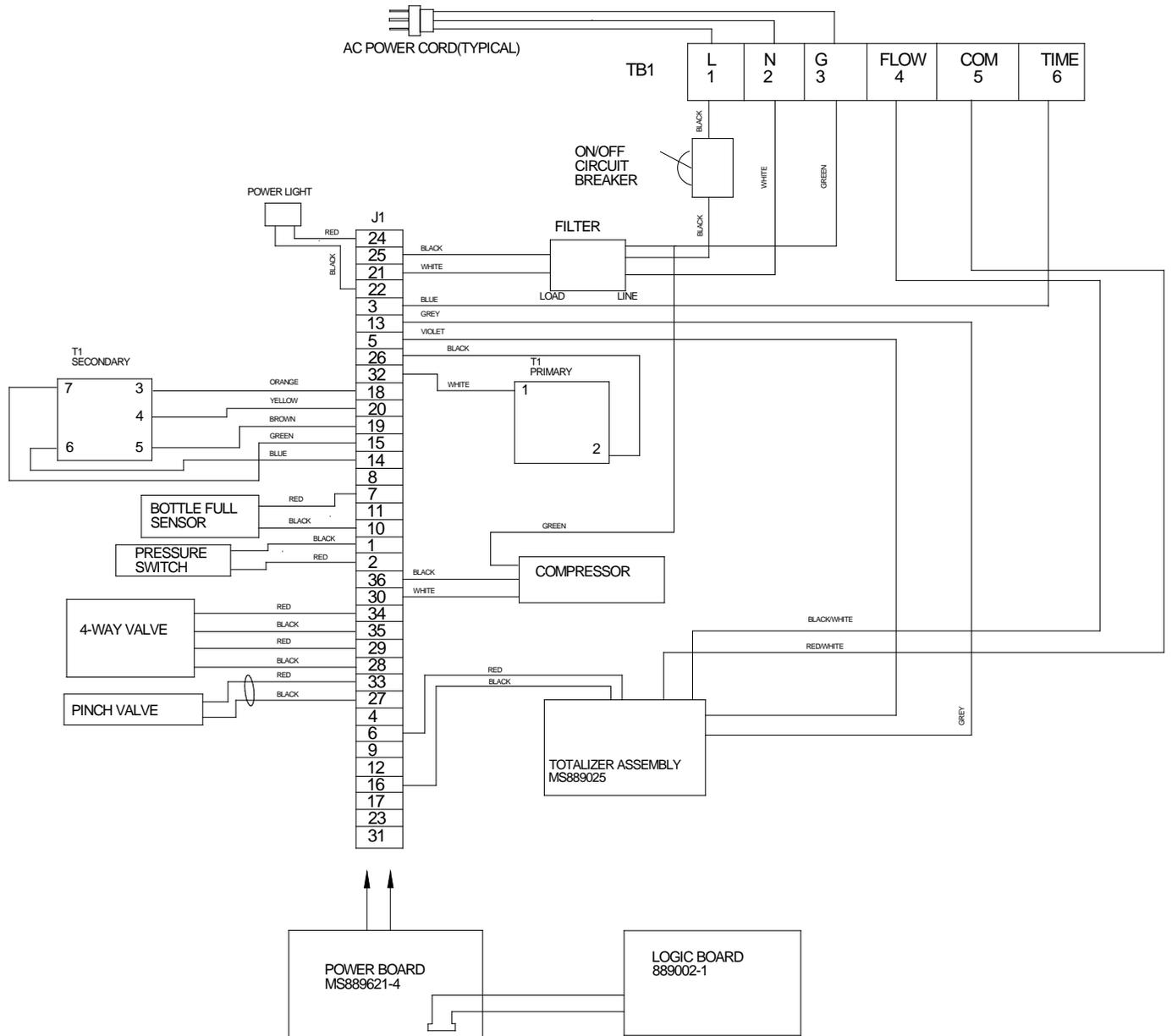
Figure 20. S-5000 Wiring Diagram with Totalizer
