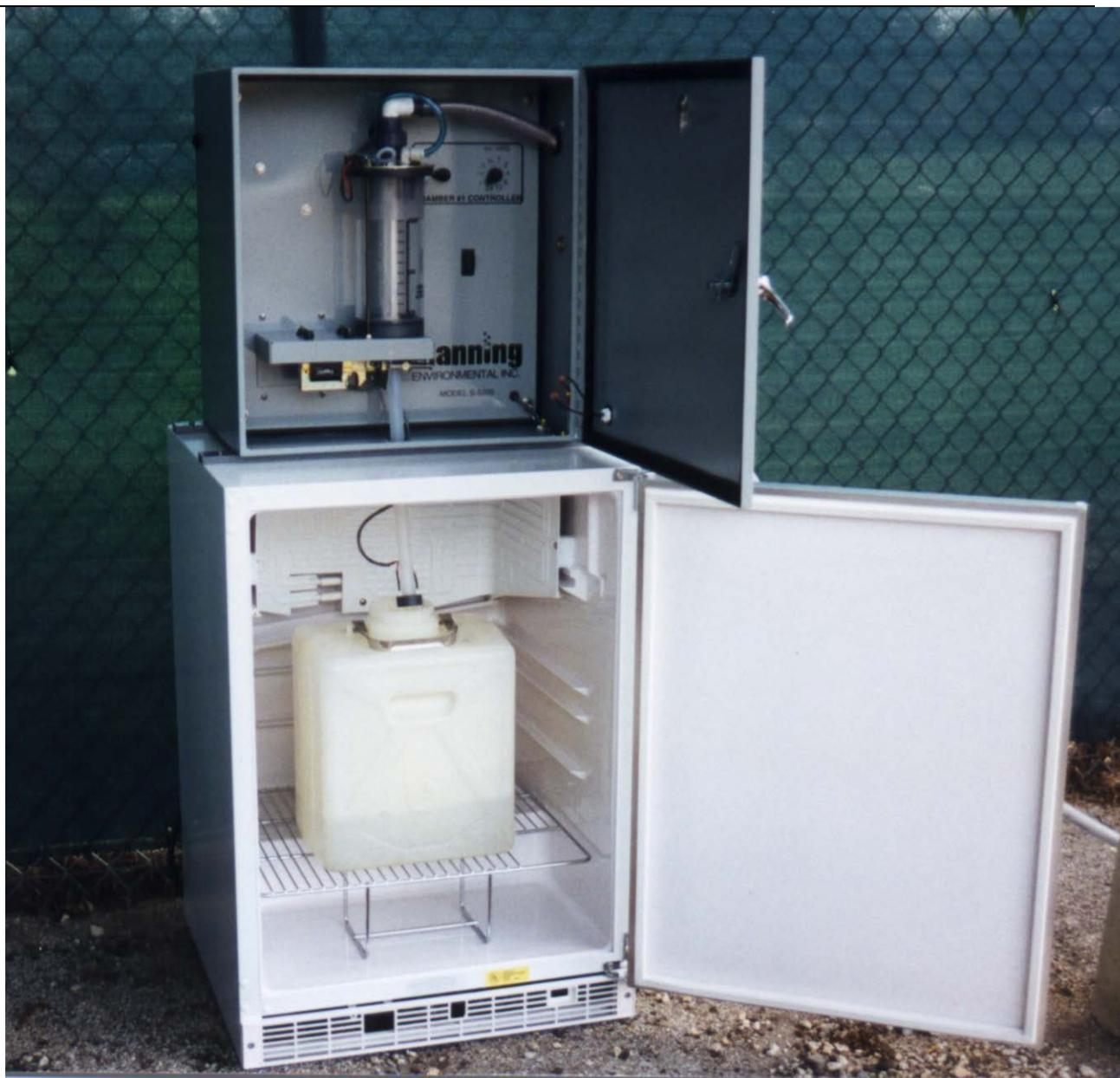
**Figure 2. S-5000 Stationary Composite Sampler, Electronics Enclosure Mounted on Refrigerator**
