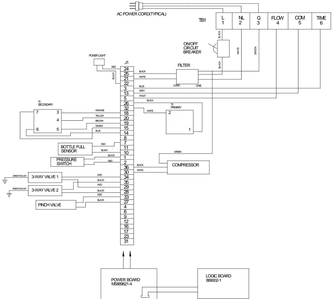
Figure 21. S5000 Wiring Diagram (Feb 2014 and Later)
