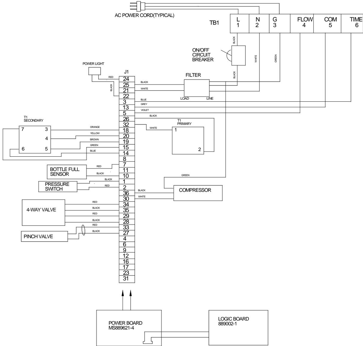
Figure 19. S-5000 Wiring Diagram (Jan 2014 and Earlier)
