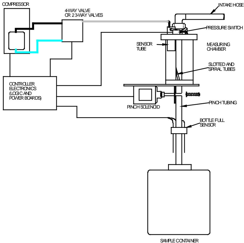
Figure 5. S-5000 Functional Block Diagram.
