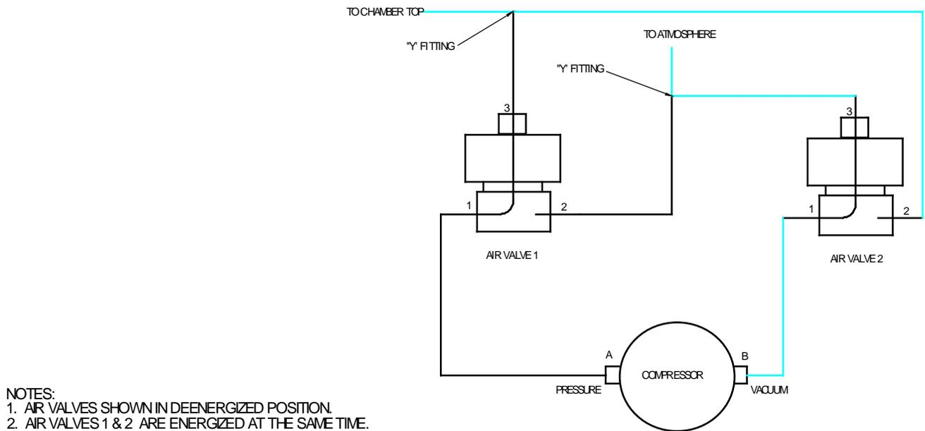
Figure 23. S-5000 Air System Diagram (Feb 2014 and Later)
