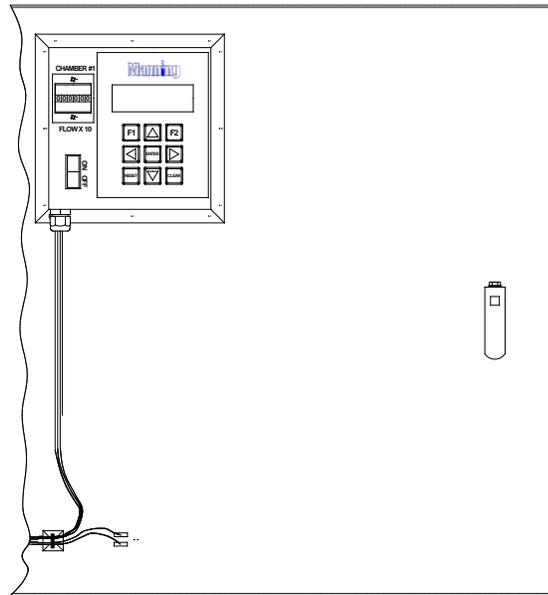
**Figure 13. Totalizer Mounted on the S-5000 Electronics Enclosure Front Door**
