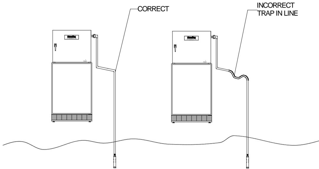
**Figure 9. Intake Hose Placement**
