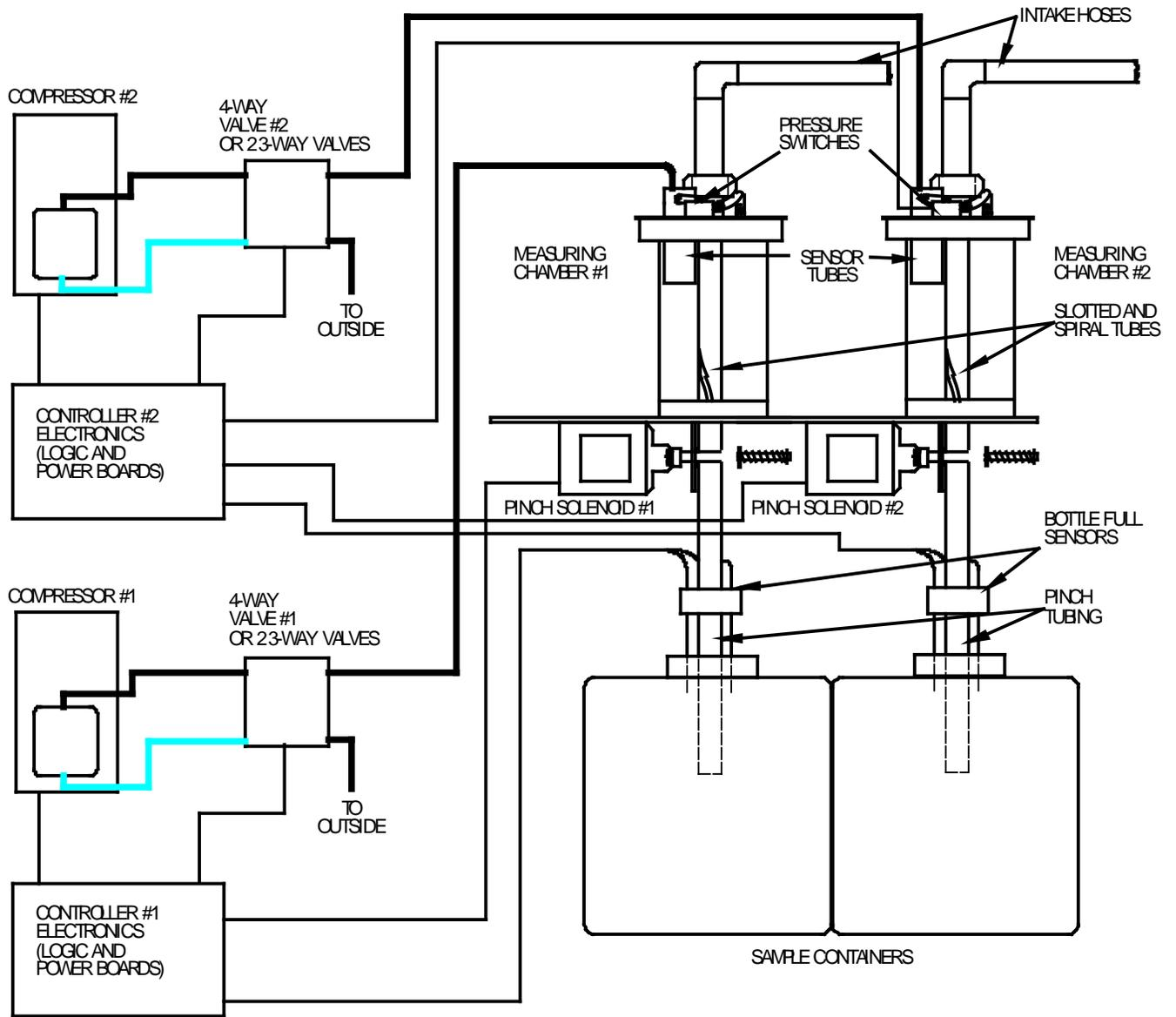
Figure 6. S-5200 Functional Block Diagram.
