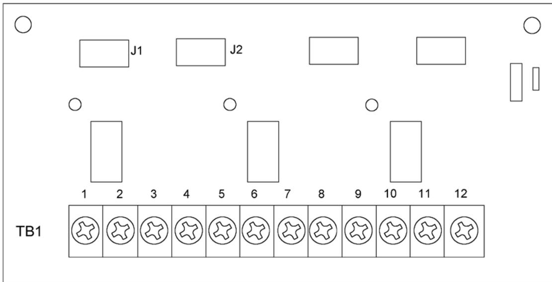
Output connections: Bottle Full- TB1-1 & TB1-2 and TB1-3 & TB1-4; Sample Cycle- TB1-5 & TB1-6 and TB1-7 & TB1-8; Missed Sample- TB1-9 & TB1-10 and TB1-11 & TB1-12
