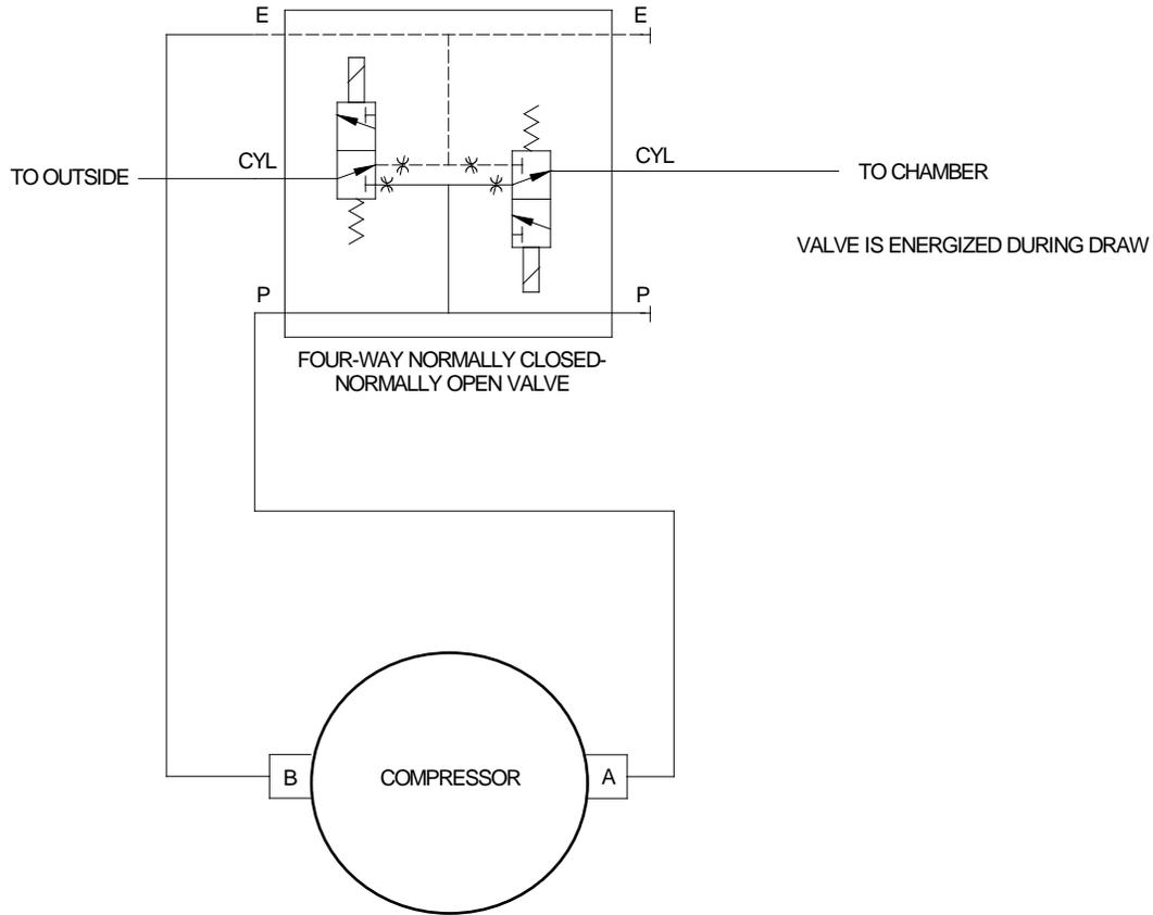
**Figure 23. S-5200 Air System Diagram
