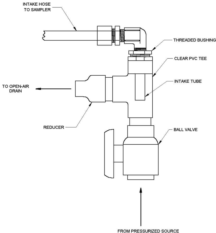
**Figure 18. Flow-Through Cell Operation**
