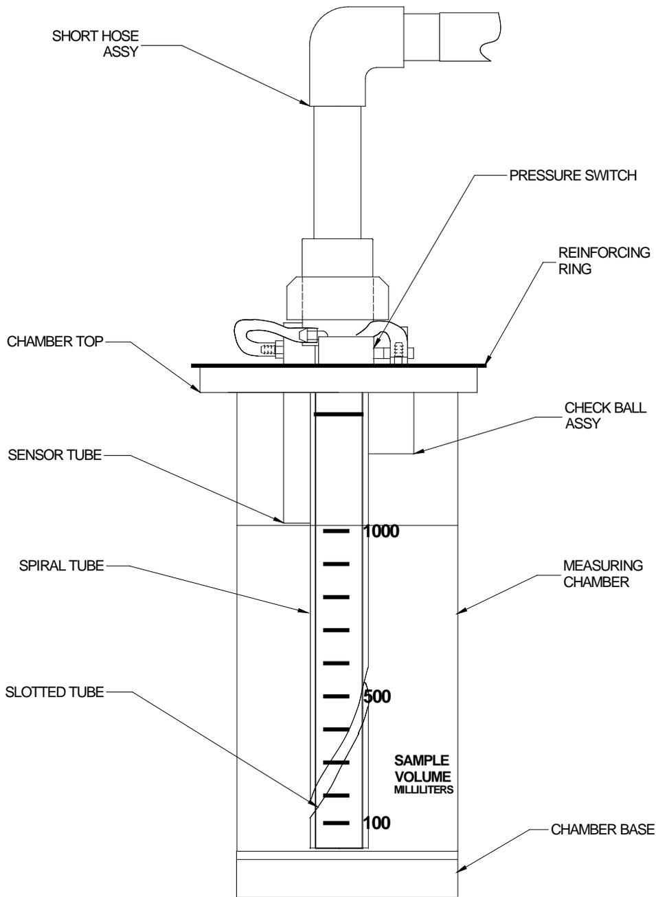
Figure 5. Measuring Chamber
