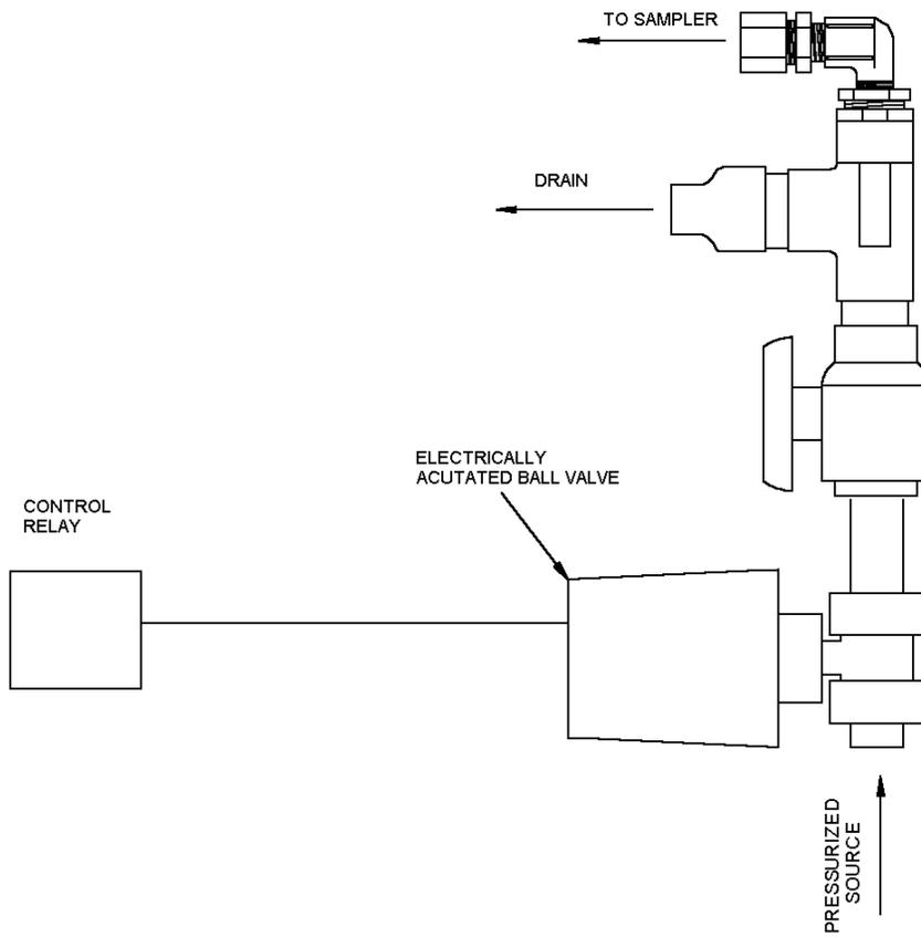
Figure 19. Flow-Through Cell with Electrically Actuated Ball Valve
