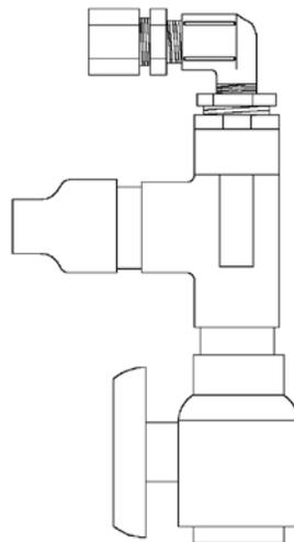
Figure 17. Flow-Through Cell
