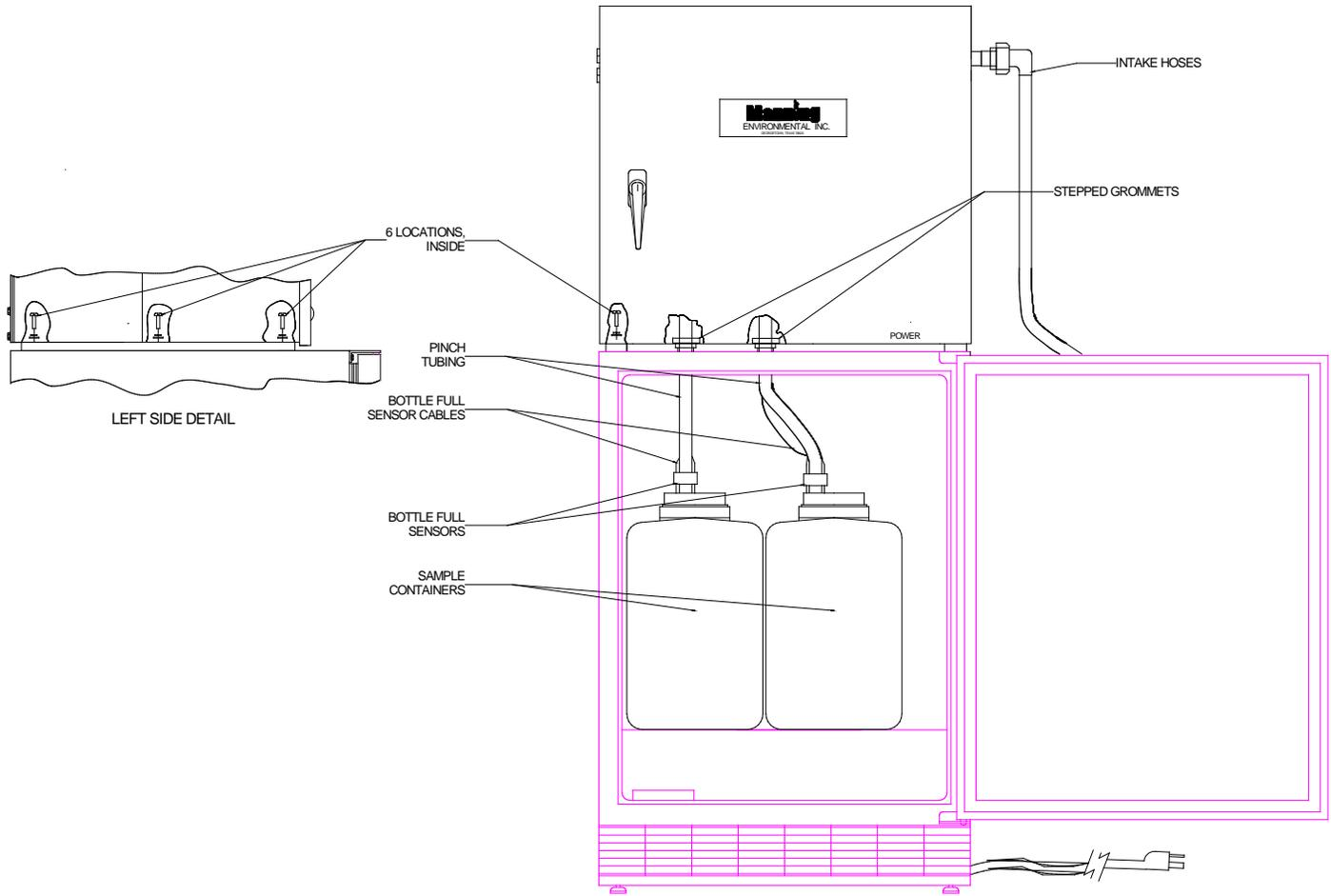
Figure 11. Model S-5200 Sampler Installation With Refrigerator
