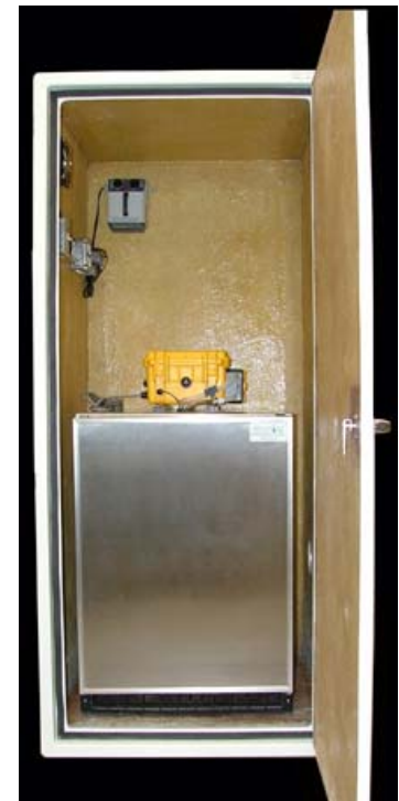
Manning YB8 Sampler in NEMA3R Enclosure
