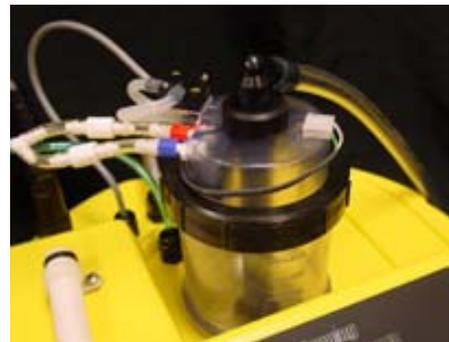
Vacuum systems also have no consumable parts that need regular replacement, and because the fluid does not travel through the pump unit, large particles or solids will not damage the sampler.
